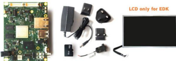
The standard Development Kits are made by one Novasom Industries board, Micro SD 4GB with SDK and SW demo, power supply wall plug, console cable, instructions to download the SDK loaded into a working Virtual Machine, for Linux OS, where **everything** is installed, **configured** and nothing additional needs to be done.
